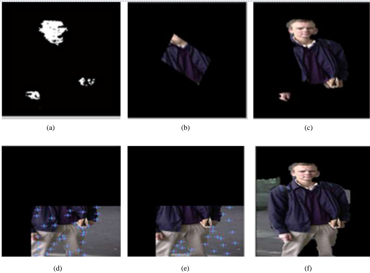
Fig.4. Simulation Results for given input. (a) Face and Skin detection, (b) Rectangular mask for upper body detection, (c) Face and Upper body Collaboration, (d) Foreground selection, (e) Background selection, (f) Final Result.
